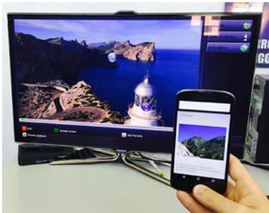
Figure 4. Prototype of the second-screen application, showing the additional information of a Point of Interest
